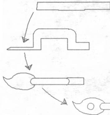
Draw out a railroad spike while preserving the original width. Form a fishtail finial & turn an eye. Wrap the eye around the hasp & curve the spike into a graceful arc bringing the spike head flat to the door plate.
