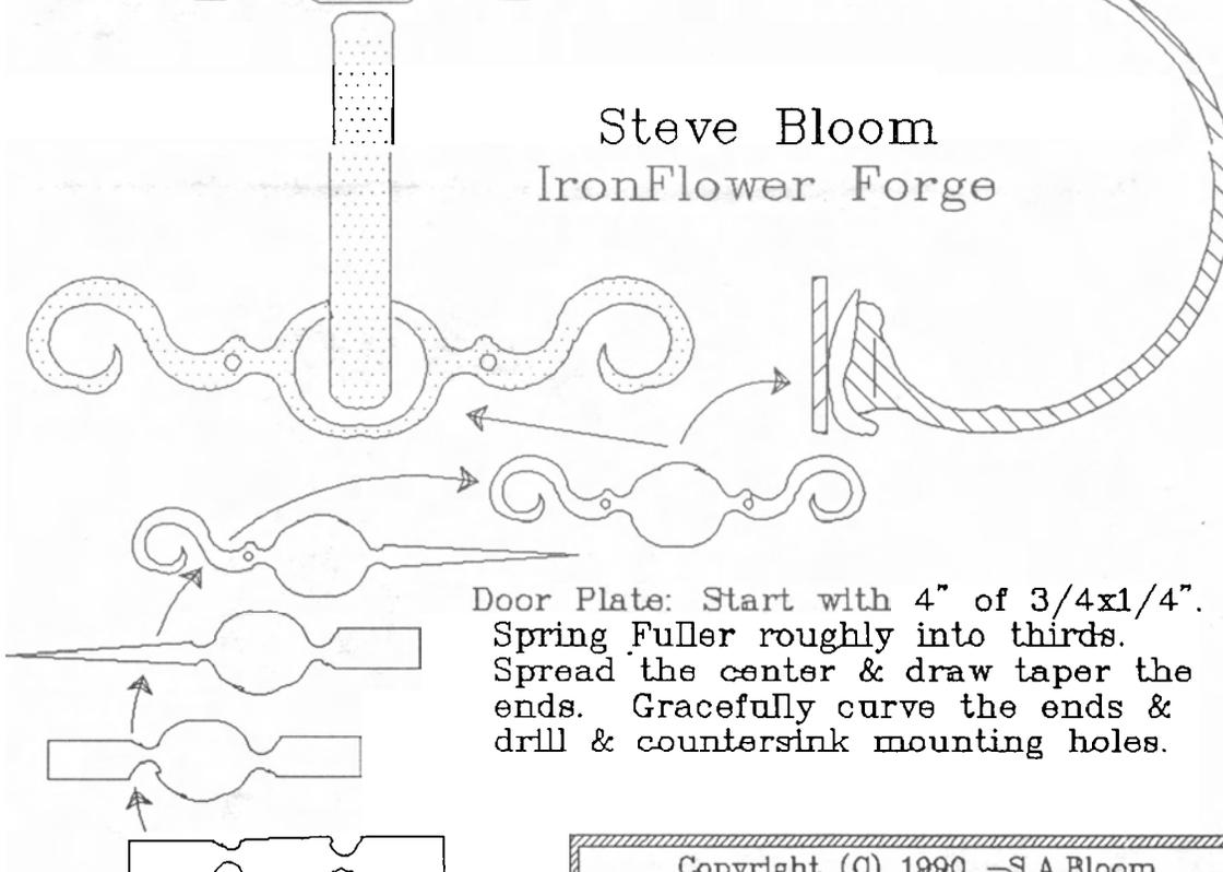
Door Plate: Start with 4" of 3/4x1/4". Spring Fuller roughly into thirds. Spread the center & draw taper the ends. Gracefully curve the ends & drill & countersink mounting holes.
